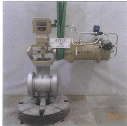
Control valve after overhaul
