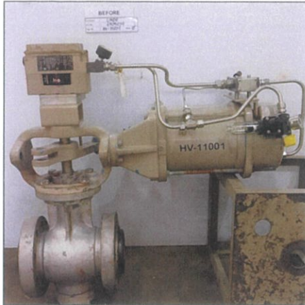
Control valve before overhaul
